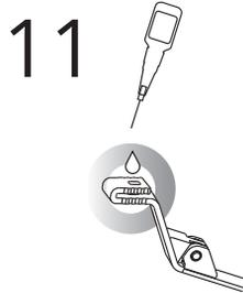
Fix the lugs and temples to the lenses, making sure the hooks are correctly inserted as shown in fig. 13, and that the temples are tilted properly to ensure the pantoscopic angle is  $7^\circ$  as shown in fig. 14. **Dry under a UV lamp for 10 seconds.**
