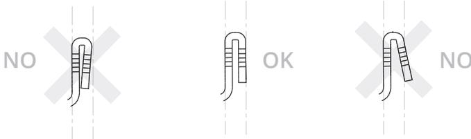
Use a needle  $\varnothing$  0.40 mm to place a small amount of glue on top of the holes on the hooks.
